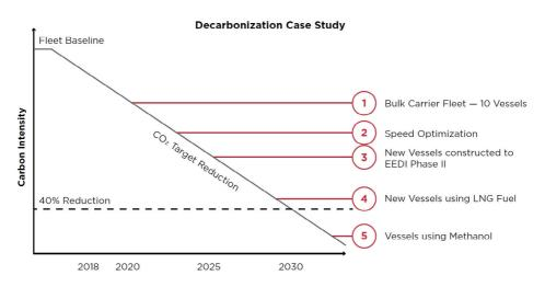
Figure 3. Decarbonization ABS Case Study Source: SETTING THE COURSE TO LOW CARBON SHIPPING, American Bureau of Shipping, JUNE 2021
