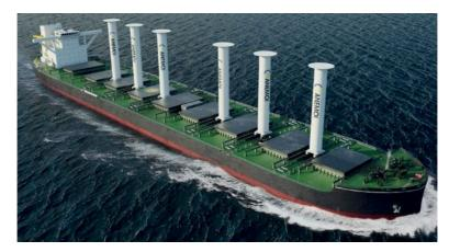
Figure 5. Newcastlemax Ship With Rotors Source: Norsepower's Rotor Sails
