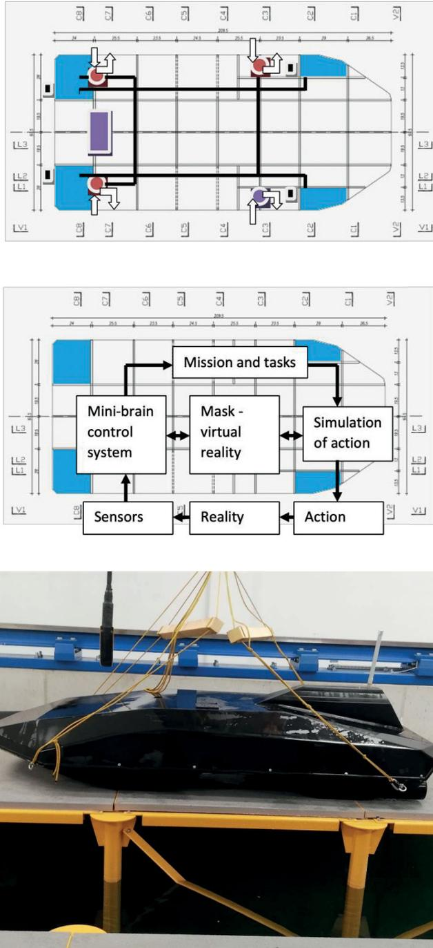
**Figure. 4.** Some elements of the AUV-AI-based control system, including the ballast system and elements of the AUV-AI-based Mask systems, also some elements of the novel USV-WIG platform system, including the AI-based control system.
