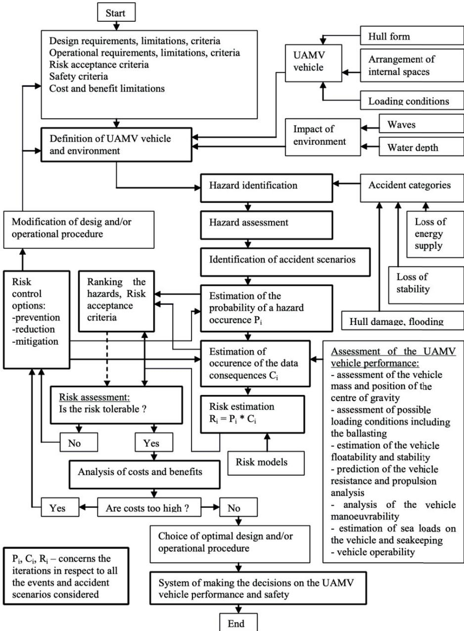
**Figure 2.** A Structure of the method for assessment of the AUV or USV-WIG vehicle performance and risk assessment (Gerigk M.K., 2014–2018).
