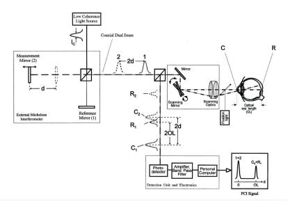
Image 7. Sketch of the partial coherence interferometer. The eye is illuminated by the interferometer, then reflected signals, for example C1, C2, R1, and R2, are superimposed on and detected by a photodetector.
