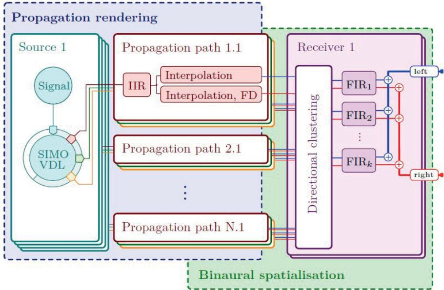
**Figure 5.** DSP network for real-time auralization of dynamic, outdoor environments. Each of  $N$  sources provides a signal that feeds a SIMO-VDL. Read cursors per source receiver pair transfer a delayed propagation path signal including spectral propagation effects.
