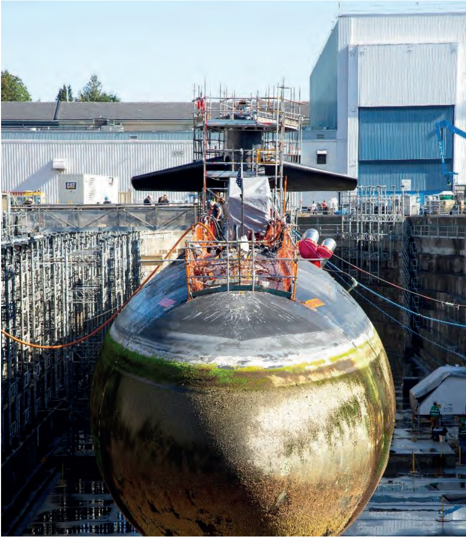
Figure 1. Biofouling on the hull of the USS Pittsburgh (SSN 720) in Bremerton, Washington, as she awaits inactivation in dry dock at Puget Sound Naval Shipyard and Intermediate Maintenance Facility. Photograph by Wendy Hallmark.
