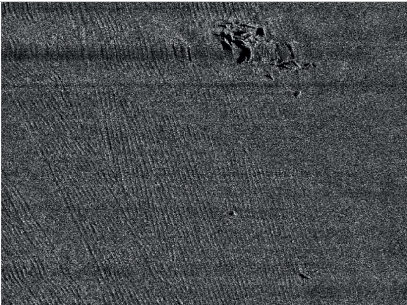
Fig. 3. A side-scan sonar image in the Western Approaches to the English Channel showing furrow lines cut by a scallop dredge boat through a rare shipwreck of c. 1670-90 (Odyssey site 35F). At a depth of 110m,[2]
