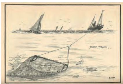
Fig. 5. Bottom beam trawling by sailing trawler around year 1850[4]. Till year 1980 weight of the trawling gear increased to 30 tons[5] .
