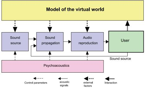
Figure 2. Implementation of an acoustic VR system
