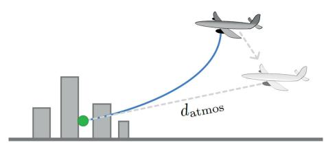
Figure 3. Definition of virtual source based on an atmospheric free field path (after Schäfer and Vorländer 2021).
