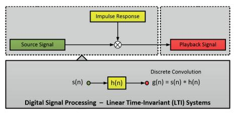
**Figure 1.** Key features of auralization: sound signal, sound propagation filter (impulse response), and sound playback.
