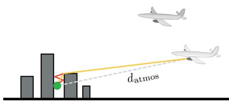
Figure 4. Atmospheric free field path (dashed, grey) and determination of urban paths (yellow and red) based on this virtual source position and an urban propagation model.
